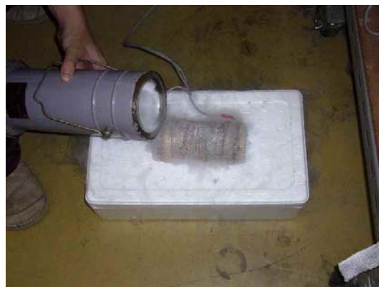
Figure 5. Cooling down of the furnace with liquid N 2 .
