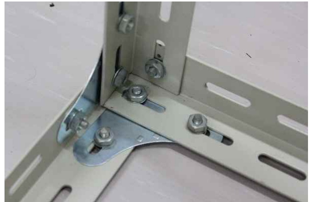
Fig. 5 The fixing of pillars and shelves using triangles.
