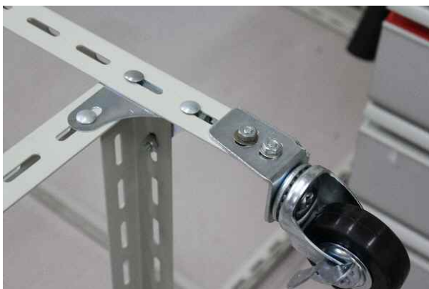
Fig. 3 The fixing of a caster to a pillar.
