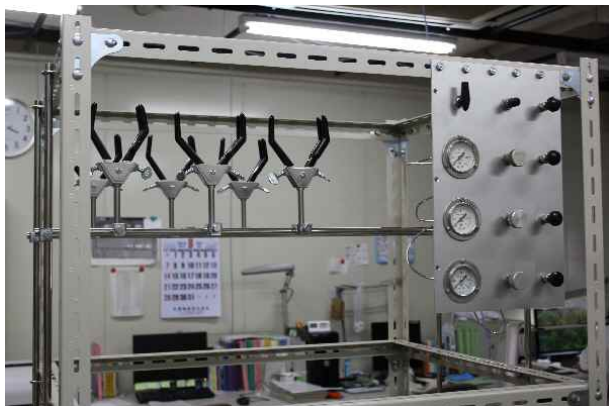
Fig. 8 The frame of the apparatus and clamps for fixing of gas cylinders made of glass.
