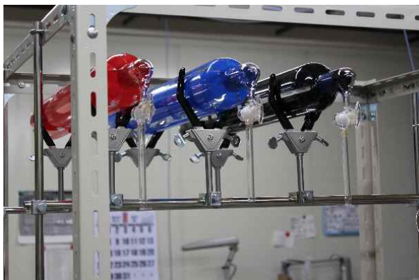
Fig. 9 The fixing of gas cylinders by clamps. The cylinders are protected by plastic tape; red is for hydrogen, blue is for carbon monoxide, black is for oxygen.
