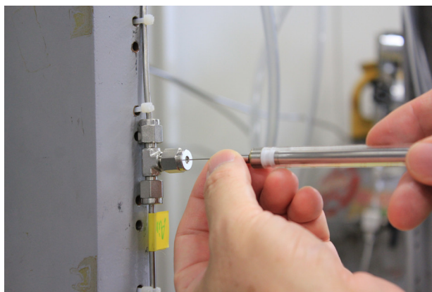
Fig. 6 Sampling of gas using a gas tight syringe.
