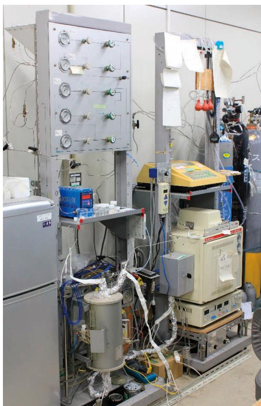
Fig. 2 Fixed-bed flow reactor system.
