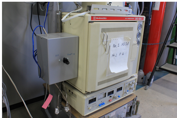
Fig. 4 The constant-temperature sampling box was connected to the gas chromatograph.
